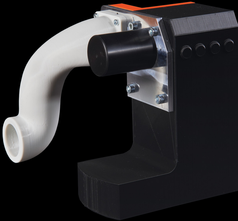
Extraction device made of PET | FFF process | Application: automation
